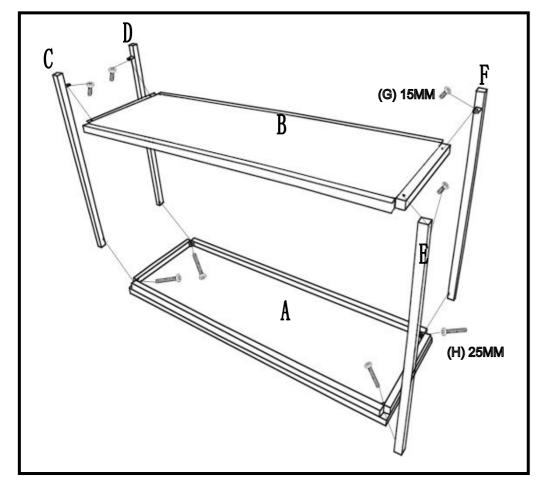
**Step 1**Attach Legs (C) (D)(E)(F) to the Table top (A), use Allen Key to tighten the long bolts (H). Then attach the Shelf (B) to the legs, tighten the short bolts (G).
