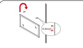
③ Install the screws into the wall anchors, leaving enough of the screw exposed to hang the mirror - approx 1/4" -1/2".
