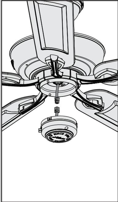
Connect the plugs from the upper and lower switch housings. Make sure to line up the colored markings on the plug connectors.
