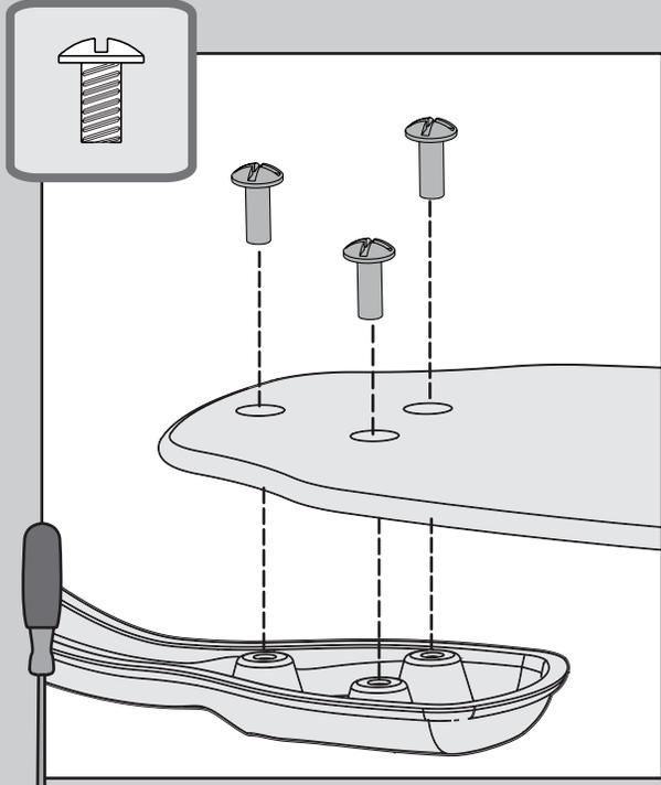
Secure each blade to a blade iron with screws found in the ▲ hardware bag.
