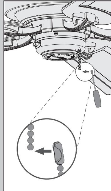
Connect the fan pull chain pendant to the short chain coming from the switch housing.
