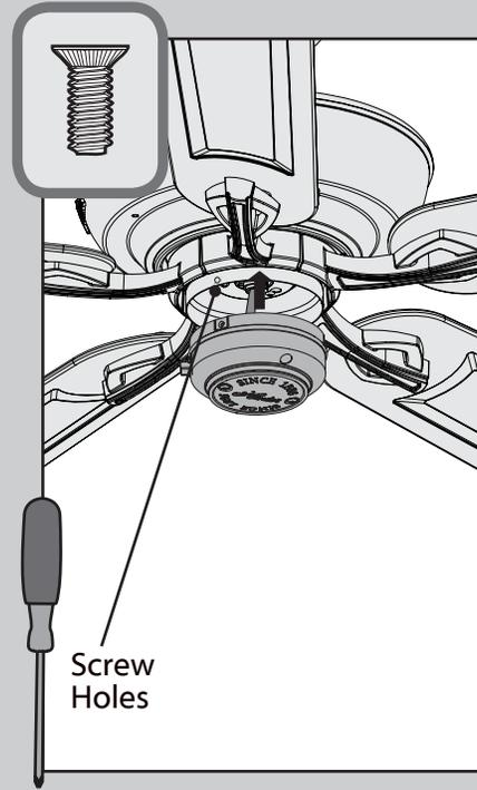
⊗ Lift the lower switch housing until the screw holes are aligned with the screw holes in the upper switch housing. Install the three switch housing screws found in the
