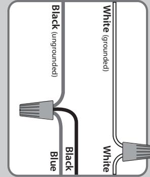
Using the orange wire connectors from the ★ hardware bag, connect the black wire (ungrounded) from the ceiling to the black and the blue wires from the fan. Connect the white wire (grounded) from the ceiling to the white wire from the fan.
