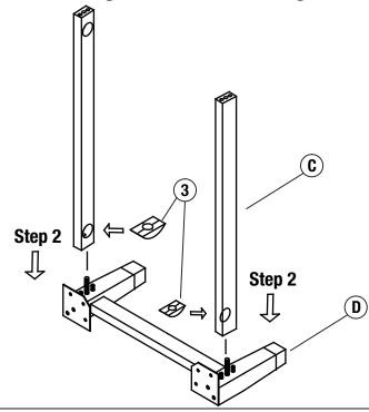
3 Installing the bottom and leg
