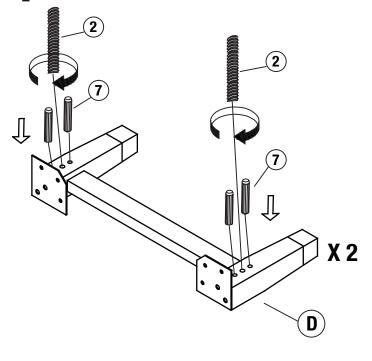
2 Installing the bottom and leg
