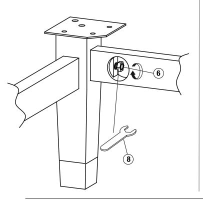
4 Installing the bottom and leg
