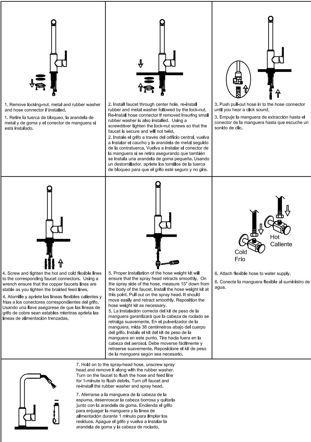
1. Remove locking-nut, metal and rubber washer and hose connector if installed.
