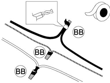
3. Strip 3/8" of insulation from the electrical wire ends. Using wire nuts (BB), connect white fixture wire to the white supply wire from the outlet box; connect the black fixture wire to the black supply wire.
