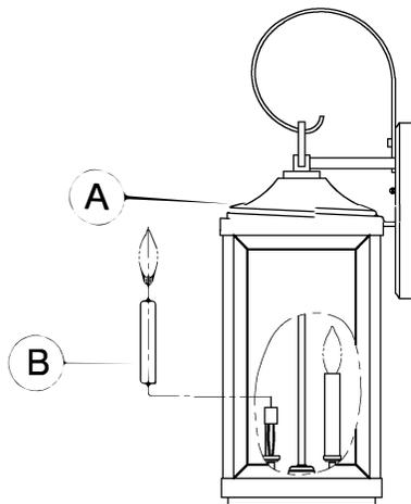
5. Attach candle covers (B) to fixture (A). Screw lamps (not included) into fixture sockets. Use 60-watt MAX incandescent candelabra base lamp, SBCFL or SBLED.
