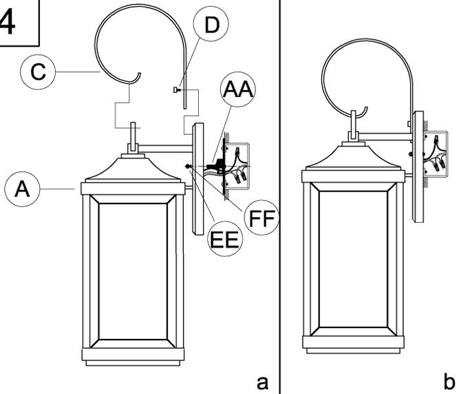
4. Put one end of the scroll (C) through the fixture (A), then attach other end to the canopy using the cylinder screw (D) to secure tightly. Install fixture (A) to screw (AA) using ball nut (EE) and waterproof o-ring (FF).
