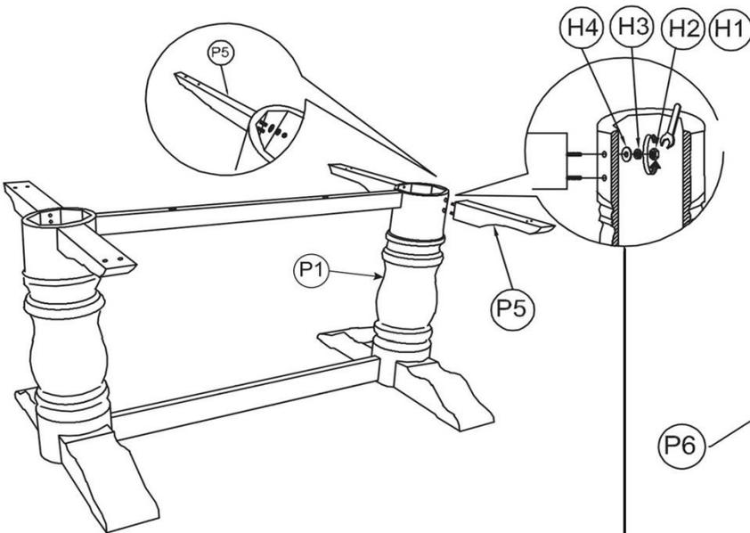
Assemble Mounting Bar P5 into the Pedestal legs P1.
