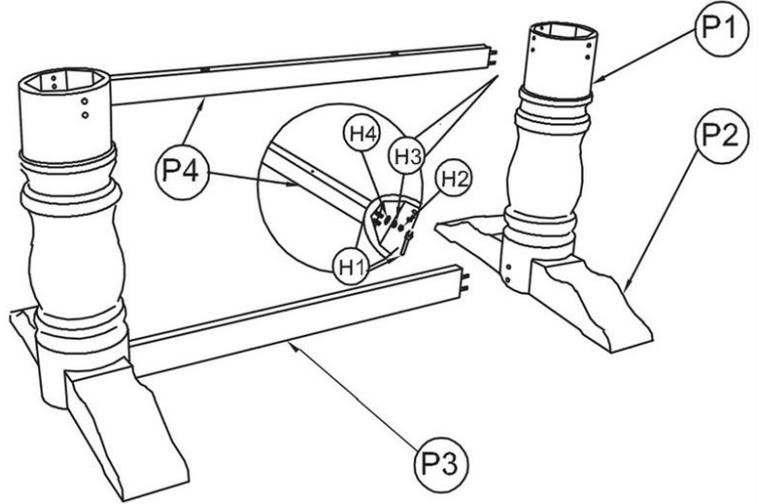
Assemble leg prongs P2 to both Pedestal Legs P1, then align Bottom Stretcher P3 and Top Rail P4 to connect both Pedestal Legs.
