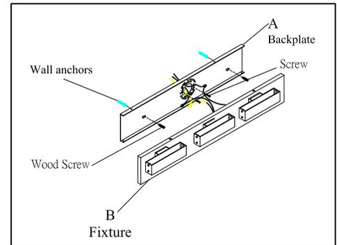
Step.1: Remove backplate (A) from fixture (B) and install to electrical box. Mark where anchors meet the wall. Drill holes using 3/16" ± drill bit where marked. Install backplate (A) to outlet box and attach anchors to secure bracket at ends.
