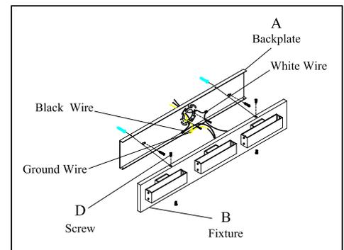
Step.2: Wire fixture to wires in outlet box. Copper wire is for Ground. Attach fixture (B) to the backplate (A) using screws (D) provided.
