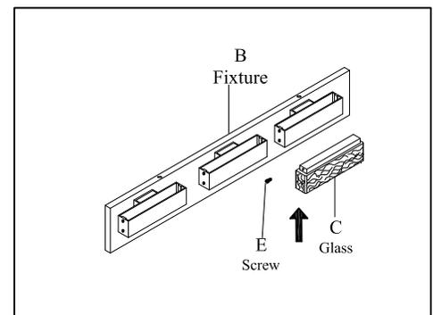
Step.3: Attach glass (C) to fixture (B) using screws (E).
