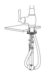
7. Once installation is complete, turn the main water supply back on from underneath your sink. Check for any leaks underneath.
