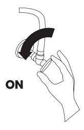
8. Turn the faucet on and ensure that there are no leaks. Check to ensure that both hot and cold water are running properly. Turn on the hand sprayer function and allow the sprayer to run for another 60 seconds, and check for any leaks.
