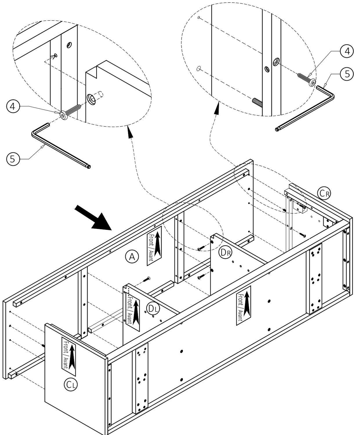
1. Attach Top (A) to Sides (CL), (CR) using six Allen Key Screws (4) ( three Screws / each Side ).
