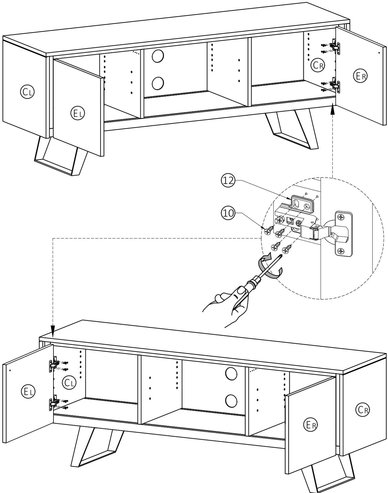
1. Attach Adjustable Hinges (12) on Doors (E) to Sides (CL, CR) using Phillips Screws (10) into guide holes on Sides (CL, CR).
