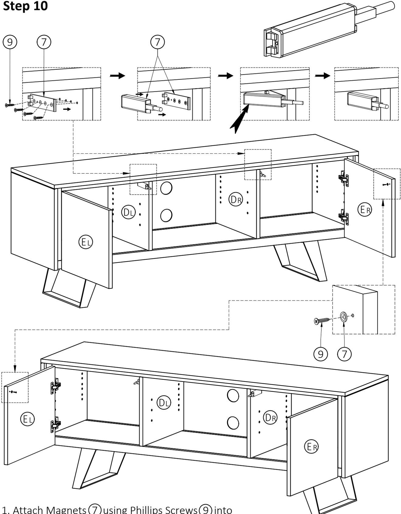
1. Attach Magnets (7) using Phillips Screws (9) into guide holes on Left Divider (DL) and Right Divider (DR).
