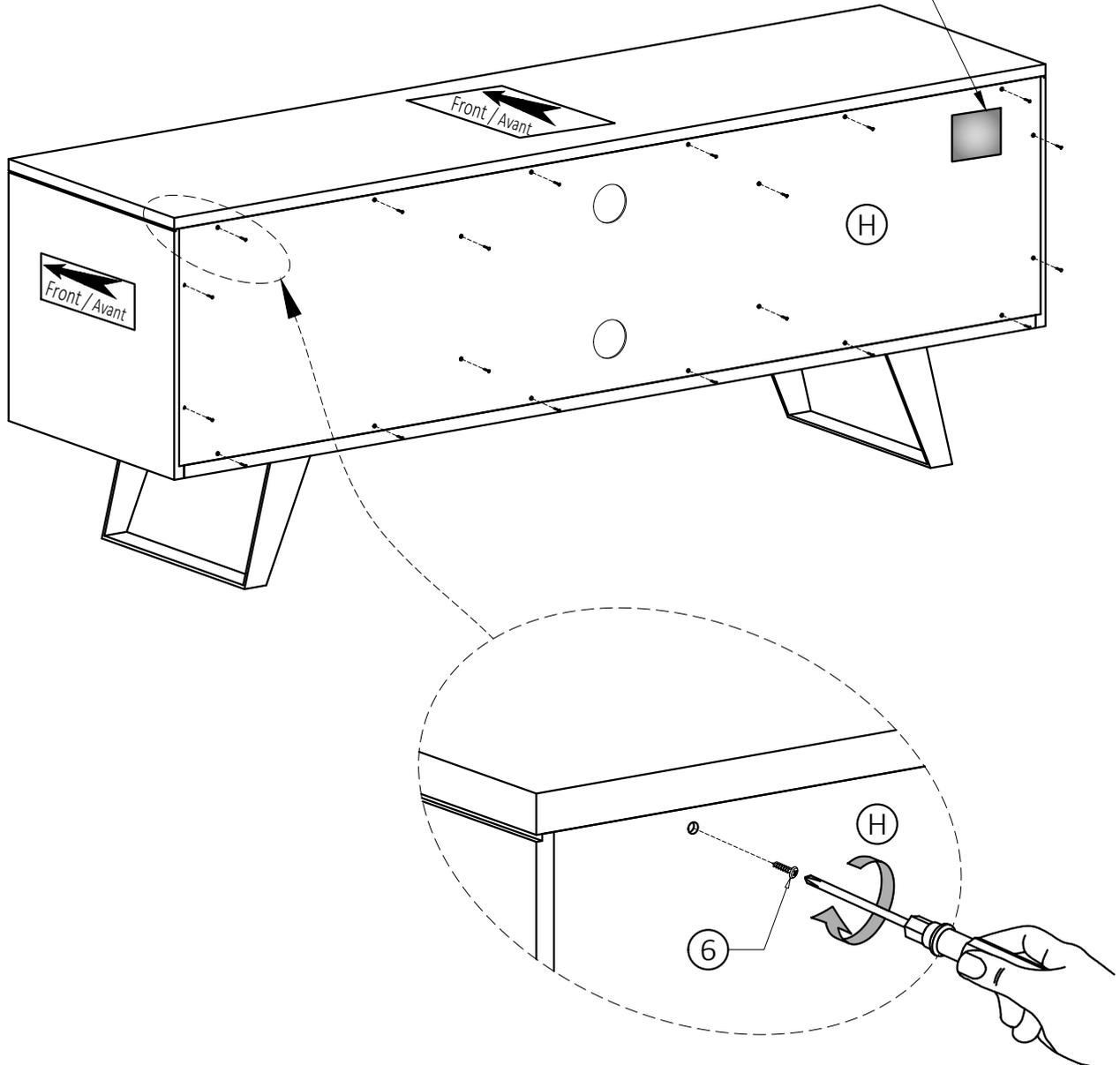
1. Attach the Top Back Panel (H) to back frame by using Phillips Screws (6).
