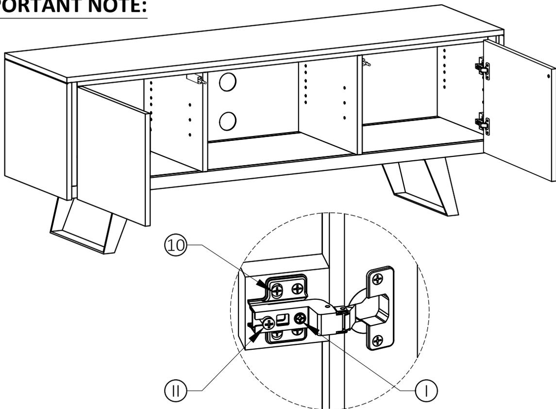
Tighten the Screw marked ⑪ to fasten hinge. The door may need to be adjusted so that all the spaces between the door and the unit sides are equal. To adjust, follow instructions:
