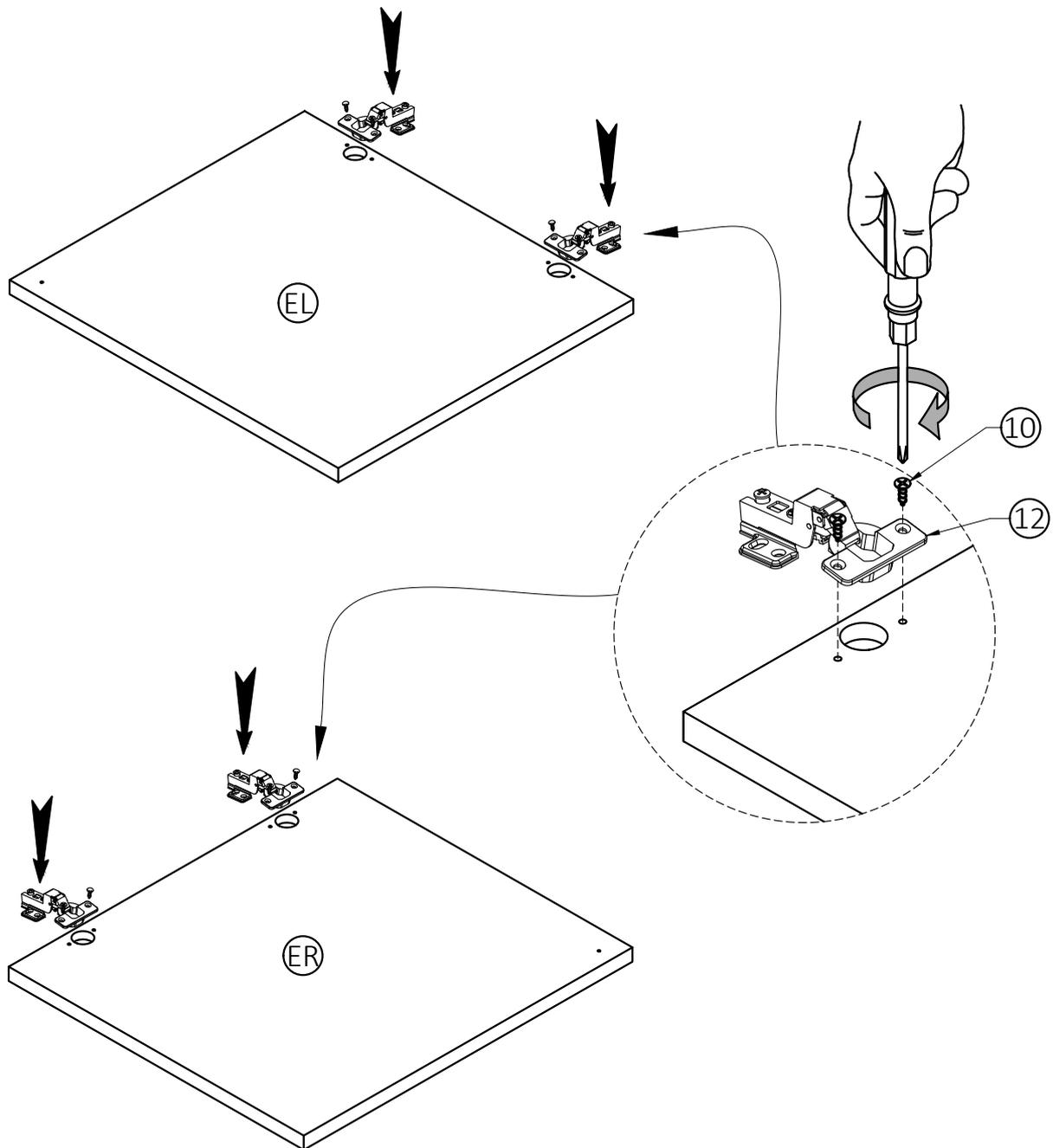
1. Attach Adjustable Hinges (12) to Doors (EL), (ER) using Phillips Screws (10) into guide holes on Doors (EL), (ER).
