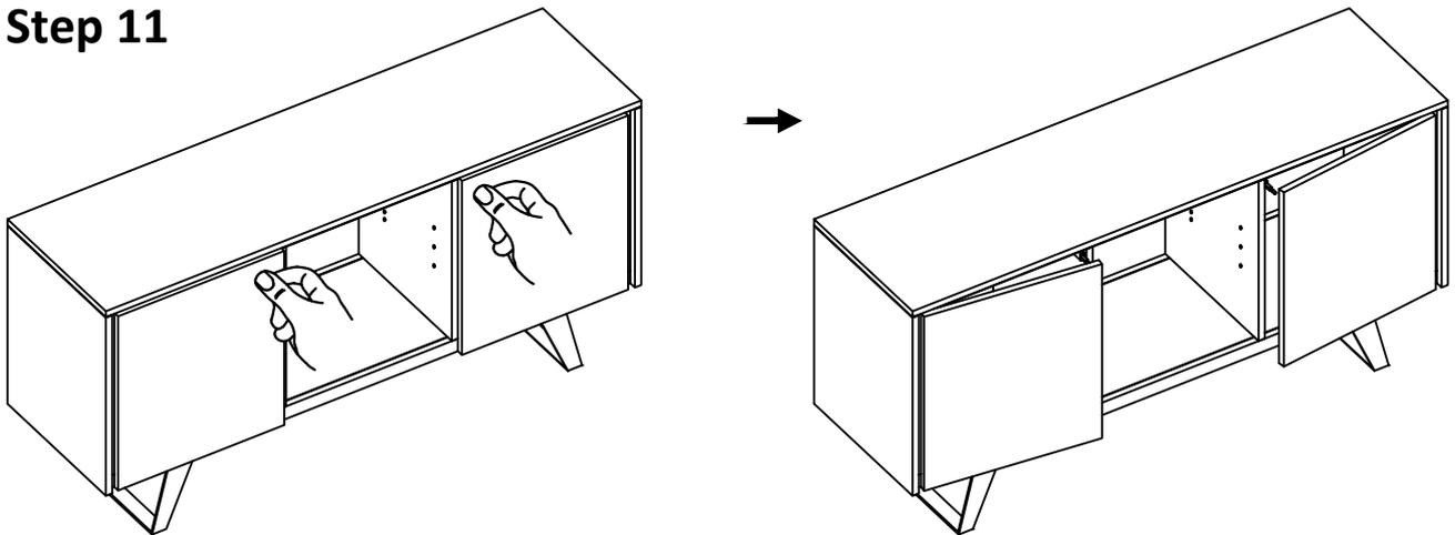
Press the top corner of the doors then release to open the doors
