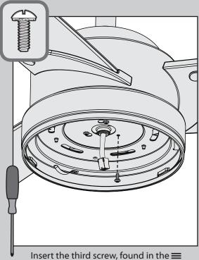
hardware bag, into place and then tighten all three screws.
