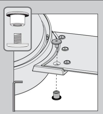
Using the included Allen wrench, secure each blade to a blade iron as shown using the blade nuts, found in the hardware bag, and the blade assembly screws, found in the hardware bag.
