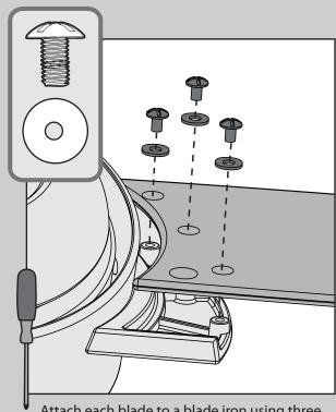
Attach each blade to a blade iron using three blade washers, found in the hardware bag, and three blade assembly screws, found in the hardware bag.
