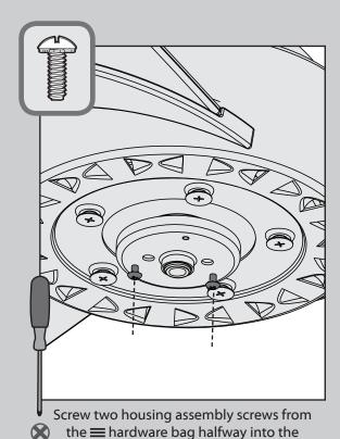
motor housing. It does not matter which
