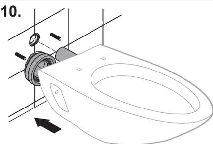
10. Before mounting bowl, measure thickness of china and mounting hardware to get approximate depth of threaded rods.
