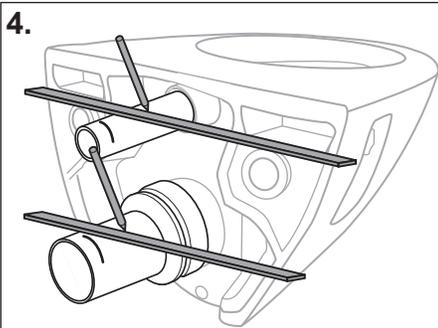
4. With a ruler, against the back of the bowl, on top of pipe, mark as shown.
