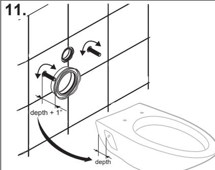
11. Use slotted end of thread bolt to adjust in or out. Do not damage the thread.
