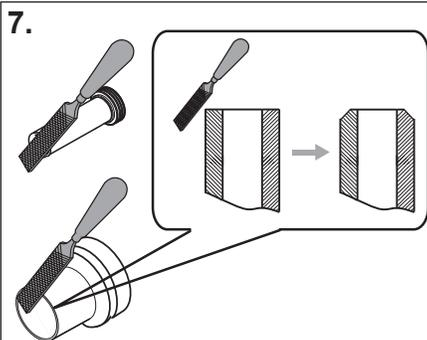
7. After cutting, take file and remove all burrs. Try and bevel edge.
