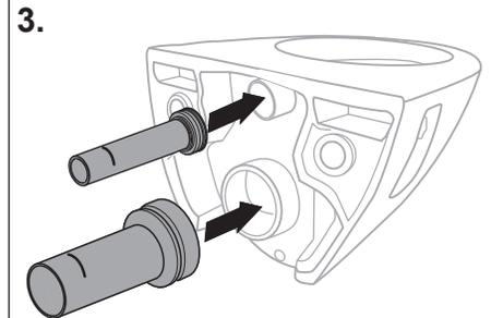
3. Remove pipes from wall and install into back of bowl. Make sure pipes are sealed thoroughly.
