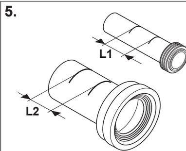
5. Measure distance between both lines on pipes. Take measured distance, deduct from bald end of pipe and cut.
