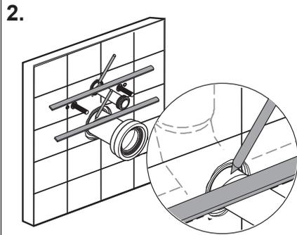
2. With a ruler, against finished wall, on top of pipe, mark as shown.
