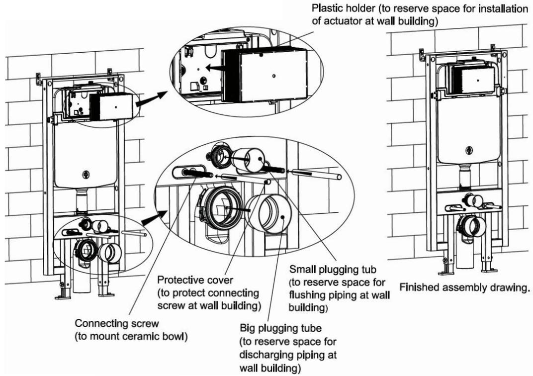
NOTE: Wall thickness ranges between 10-60mm (from outer surface of cistern to the finished wall)
