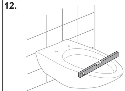
12. Install with mounting hardware and ensure toilet bowl is level.
