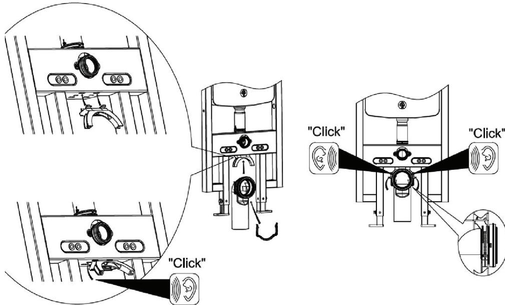
d.) After the waste pipe is secure, you may adjust the feet of the frame accordingly to properly fit the height of the waste pipe. Using a wrench, secure legs at the desired height as shown below.
