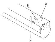
Connect wiring as shown. Gray and purple wiring are for 0-10V dimming systems. Cap off if not used.
