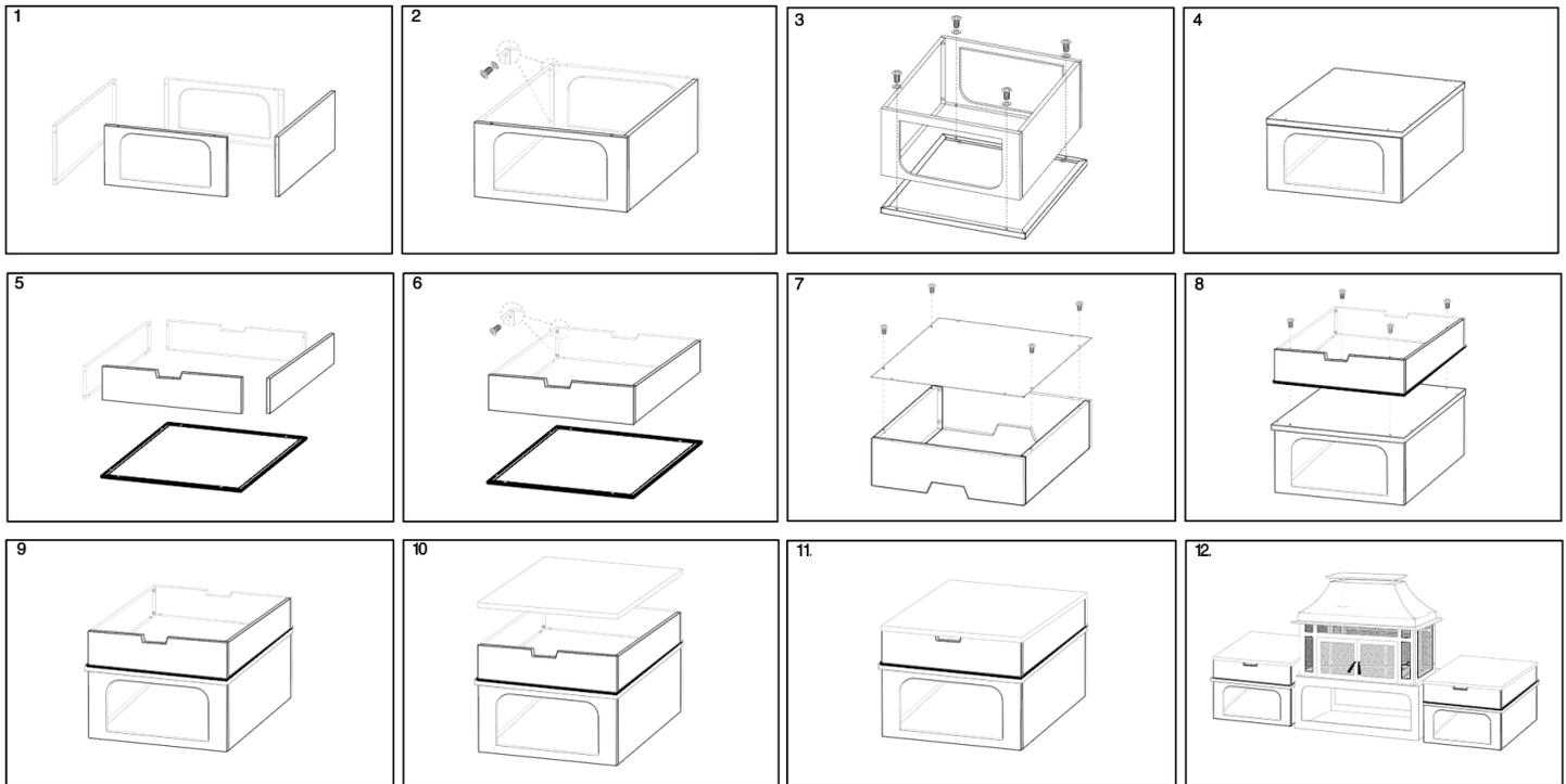
First assemble the lower section of the side storage units. It is easier to first lightly turn the screws just to hold the unit together, go back after to tighten all in place. Lay the flat sheet with the U channel edges up-side-down on a section of the packing
