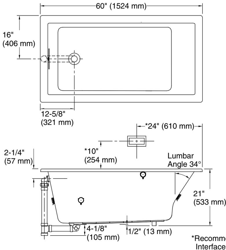
No change in measurement if connected with drain illustrated. (K-7272)
