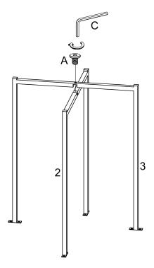
Attach part (3) to part (2) using bolt (A) with hex key (C).
