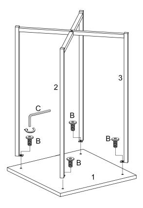
Attach part (2,3) to part (1) using bolt (B) with hex key (C).
