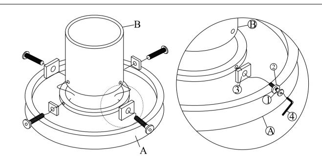
STEP 1: Tight the bolts to press with plastic plug on concrete base without piercing
