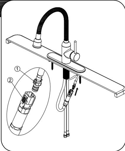
Screw quick connect assembly to the free end of hose. Align male fitting (1) and tabs (2) on quick connector. Push quick connector housing firmly upward and snap onto receiving male fitting. Pull down moderately to ensure connection has been made.
