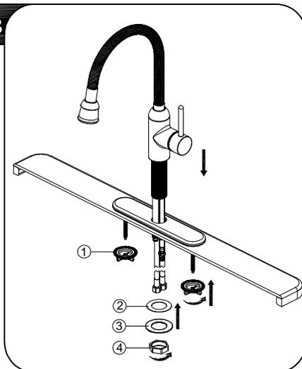
Insert faucet body through the hole in escutcheon. From underneath sink, hand tighten mounting nuts (1). Install plastic washer (2) and metal washer (3) onto the threaded mounting shank. Thread nut (4) onto mounting shank. Do not overtighten.
