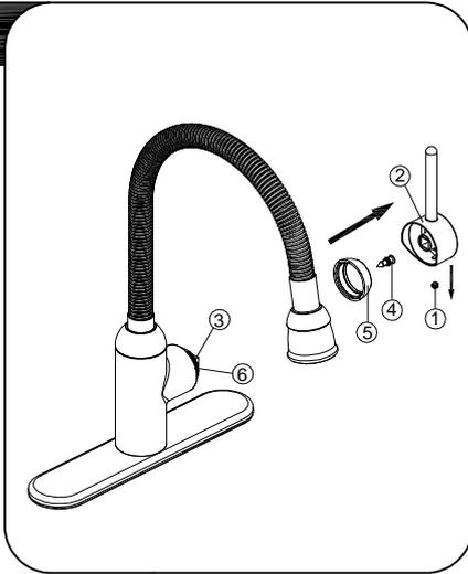
Shut off water supply. With valves in "closed" position, Loosen the set screw (1). Remove handle (2) from valve stem (3). Loosen the screw (4) from valve stem (3) and unscrew the cap (5) from the cartridge nut (6).
