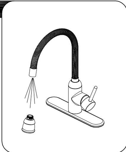
Important: after installation is completed, turn on hot and cold water supplies. Check for leaks. Remove the spray head by unscrewing it from the hose counterclockwise. Turn the faucet on to the warm position where it mixes hot and cold water. Flush water lines for one minute. Check for leaks. Re-tighten any connections if necessary, but do not overtighten. Reinstall spray head by hand tightening it back onto the hose.
