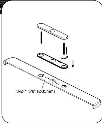
Before installation, screw bolts to the large escutcheon. Insert escutcheon assembly through the gasket and the holes of the sink.
