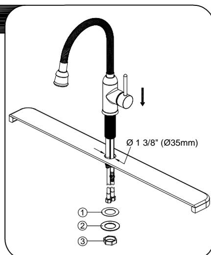
Insert faucet body through the hole in sink. Install plastic washer (1) and metal washer (2) onto the threaded mounting shank. Thread nut (3) onto mounting shank. Do not overtighten.
