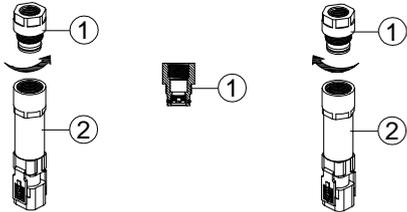
This faucet ships with a 1.5 GPM flow restrictor installed. An optional 2.2 GPM flow restrictor is also included in the box.
