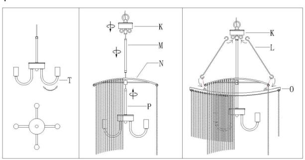
Step A1 » Adjust arms (T) to proper position as shown in the illustration.
