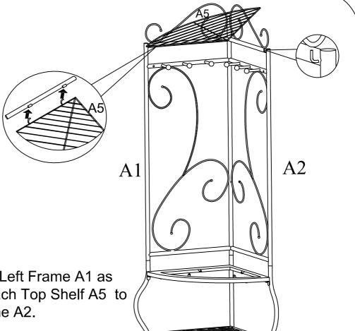
Attach Top Shelf A5 to Left Frame A1 as shown above, then Attach Top Shelf A5 to the hook on Right Frame A2.
