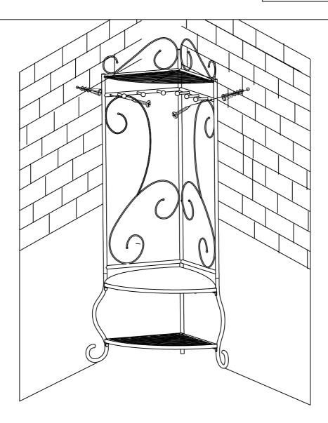
For your safety, please fix the corner hallway bench to the wall by Anchors and Screws B4.
