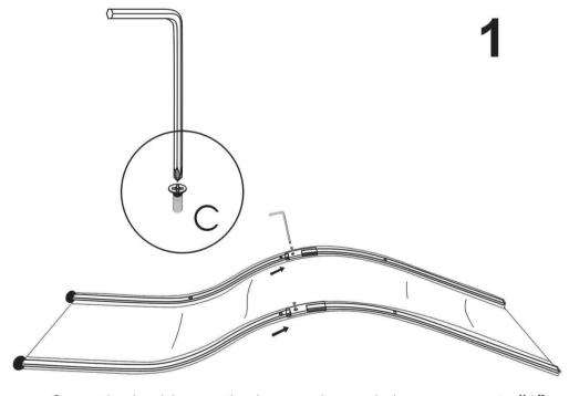
Open the bed, insert the inner tube and close screw at "1"
