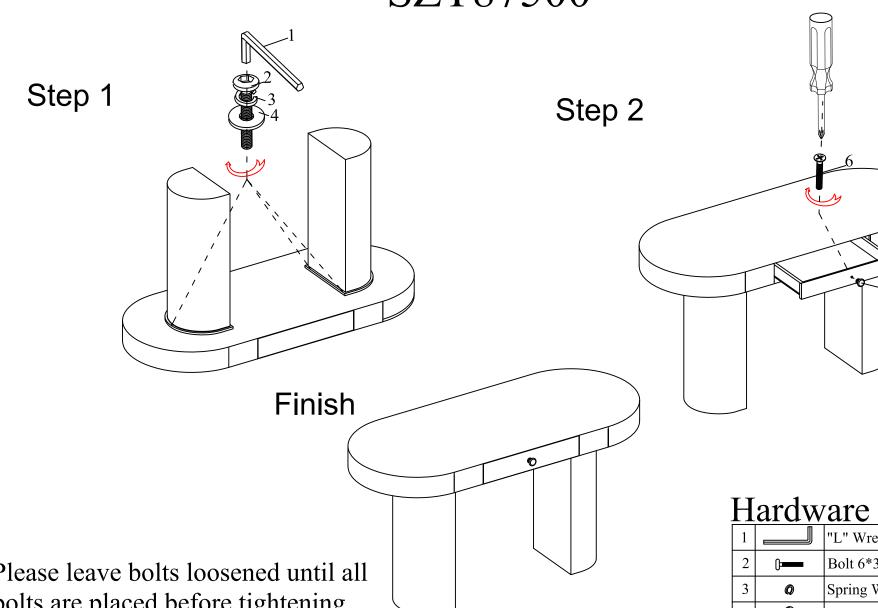
Please leave bolts loosened until all bolts are placed before tightening completely
