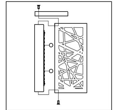
Step 3: Install fixture to back-plate and tighten worm screws so that fixture meets the wall.
