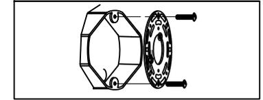
Step 1: Remove mounting bracket from fixture and install it to electrical box.
