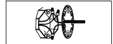
Step 2: Wire fixture to wires in outlet box. Green wire is for ground.
