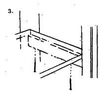
Pull both sets of legs back and fit the frame. Once in place secure the frame with the serews 54 to fully tighten.
