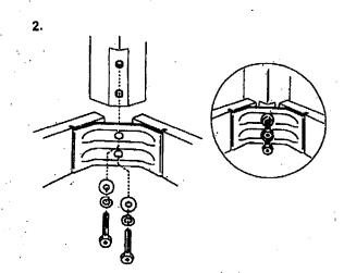
Lay the table top face down on your work surface using scrap packaging to protect the table top. Position the legs to the brackets and secure with bolts 51, spring washers 52 & washers 53.
