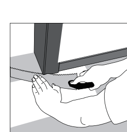
12 Door molding and skirting: lay a board (with the decorative side down) next to the door molding and as shown in the figure. Then slide the floorboard under molding.
