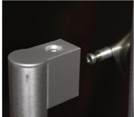
4. Hold the handle firmly against the door, make sure there are no gaps between the handle end caps and the door, and tighten both set screws in the handle end caps.
