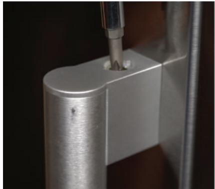
5. Place the screw caps over the set screws on the handles.
