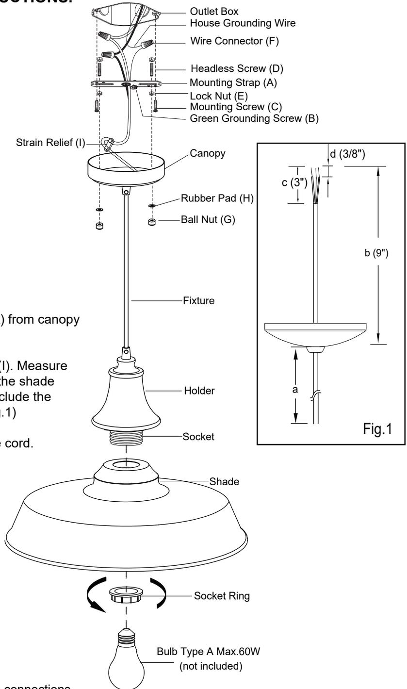
8. Pull the cord (a) down slightly until the strain relief (l) touches the hex nut. Attach the canopy to the mounting strap (A) by inserting two headless screws (D), adjust the length of the headless screw (D) if necessary. then secure it with two rubber pads (H) and two ball nuts (G).
