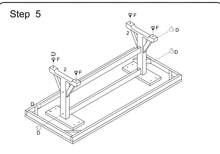
Place wood button (D) and insert adjuster (F) into legs (2) as per diagram.
