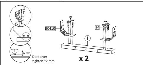
**STEP6**: Now let's combine the bottom skirt. Start with installing Corner Brace (HW BC410) into Bottom Skirt 2 (I) using Screw M4x16mm (HW14). Do not overtight screw yet, leave around 2mm gap.
