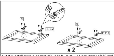
**STEP3**: Install remaining part of Hinge (HW HS35A) into Door Left (J) and Door Right (K) position as shown in picture. Secure with screws M4.5x12.5mm (HW9).
