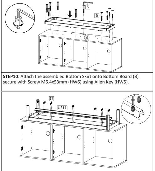
**STEP12**: Place Anti-Deflection Bar (HW US11), secure with screw M6x12.5mm (HW17), tighten using screwdriver.
