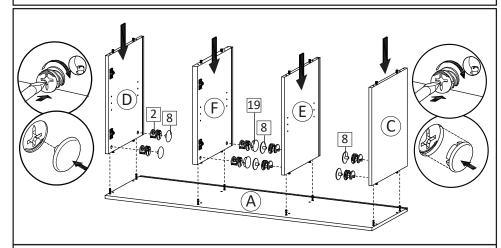
**STEP4**: Attach Side Boards (C&D) and Center Boards (E&F) into Top Board (A). Insert the Camlock (HW2) then tighten using a screwdriver. Place the Screw Caps (HW8&HW19) over the camlock as shown.
