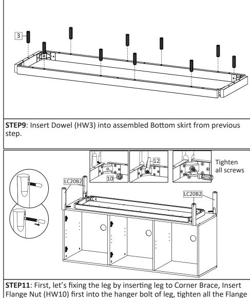
Flange Nut (HW10) first into the hanger bolt of leg, tighten all the Flange Nut using provided Wrench (HW12). Second, after Ensuring that all legs has been tightened, continue with tighten all screws on the corner brace.
