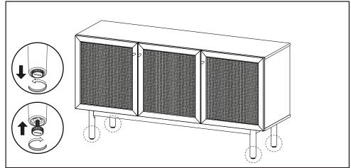
**STEP16**: Place your furniture on lever floor. The legs come with adjustable leveler, adjust it as needed until your furniture stands steadily on the floor. Assembly is Complete.
