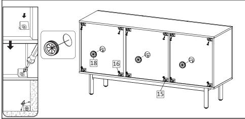
**STEP15**: Use Wedge (HW15), Screw M3.5x15.5mm (HW16) to tighten the back of media stand by using screwdriver. Please align the top board and bottom board in  $90^{\circ}$  position against the side board, before securing the wedges (HW15). Insert Hole Cable (HW18) as shown in picture.
