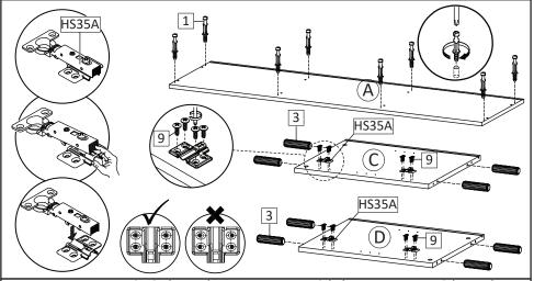
**STEP1**: Insert Cambolt (HW1) into Top Board (A). Insert Dowel (HW3) into Side Boards (C&D). Prepare Hinge (HW HS35A),Remove the Mounting Plate by pressing the backside of Hinge (HS35A). Install Mounting Plate with Screw (HW9) on Side Boards (C&D). Set aside and indicate the remaining part of the hinge as (HW HS35A) to avoid any mix up.
