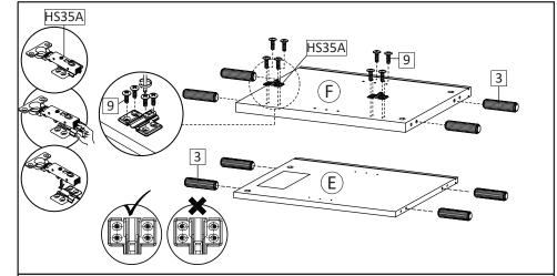
**STEP2**: Insert Dowel (HW3) into Center Board (E&F). Prepare Hinges (HW HS35A),Remove the Mounting Plate by pressing the back of the Hinge (HW HS35A). Attach the Mounting Plate with M4.5x12.5mm Screws (HW9). As shown in Step 1.
