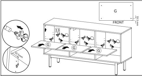
**STEP13**: After bringing the product upright, insert Shelf Support (HW13) into the holes on Side board & Center board, on the desired level. Then place the Adjustable Shelf (G) by inserting the hole on the shelf into the shelf support.
