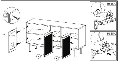
**STEP14**: Install Door Left (J) and Door Right (K) into Side Board Left,Side Board Right and Center Board. Please review above images carefully. Insert Handle (HW11) Secure with Screw M4x25mm (HW7) into Doors. Refer to separate page to adjust hinges.
