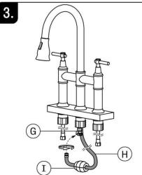
3. Put the pull tube (H) into the water outlet (G). Then put the gravity ball (I) on pull tube and adjust it in right position. Prepare the next step.
