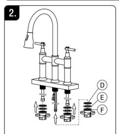
2. Use a nut (F) to fix the faucet. Rubber washer (D) and metal washer (E) are needed between the nut and fixed plate.
