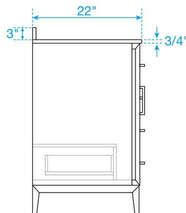
\*Note: Due to high probability of breakage, the backsplash comes in two pieces, cut from the same piece. All measurements are  $\pm$  1/4".
