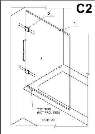
3. Remove the door and drill holes into the wall where marked. Place plastic anchors (#7) inside the holes.
