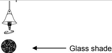
Install the glass on the lampholder, Do not over tighten.
