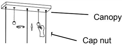
Attach the canopy to the mounting plate with screws provided.
