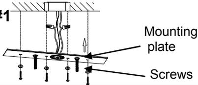
Attach the mounting plate to junction box with screws.
