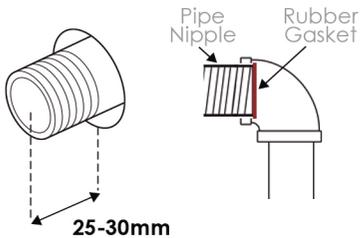
Pipe Nipple Rubber Gasket
