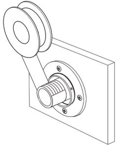
Wrap the exposed threaded area of the pipe with Teflon tape.
