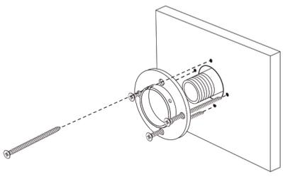
After inserting wall anchors, secure the mounting ring with the provide screws. Ensure the screws are positioned to avoid interference with the piping behind the wall.
