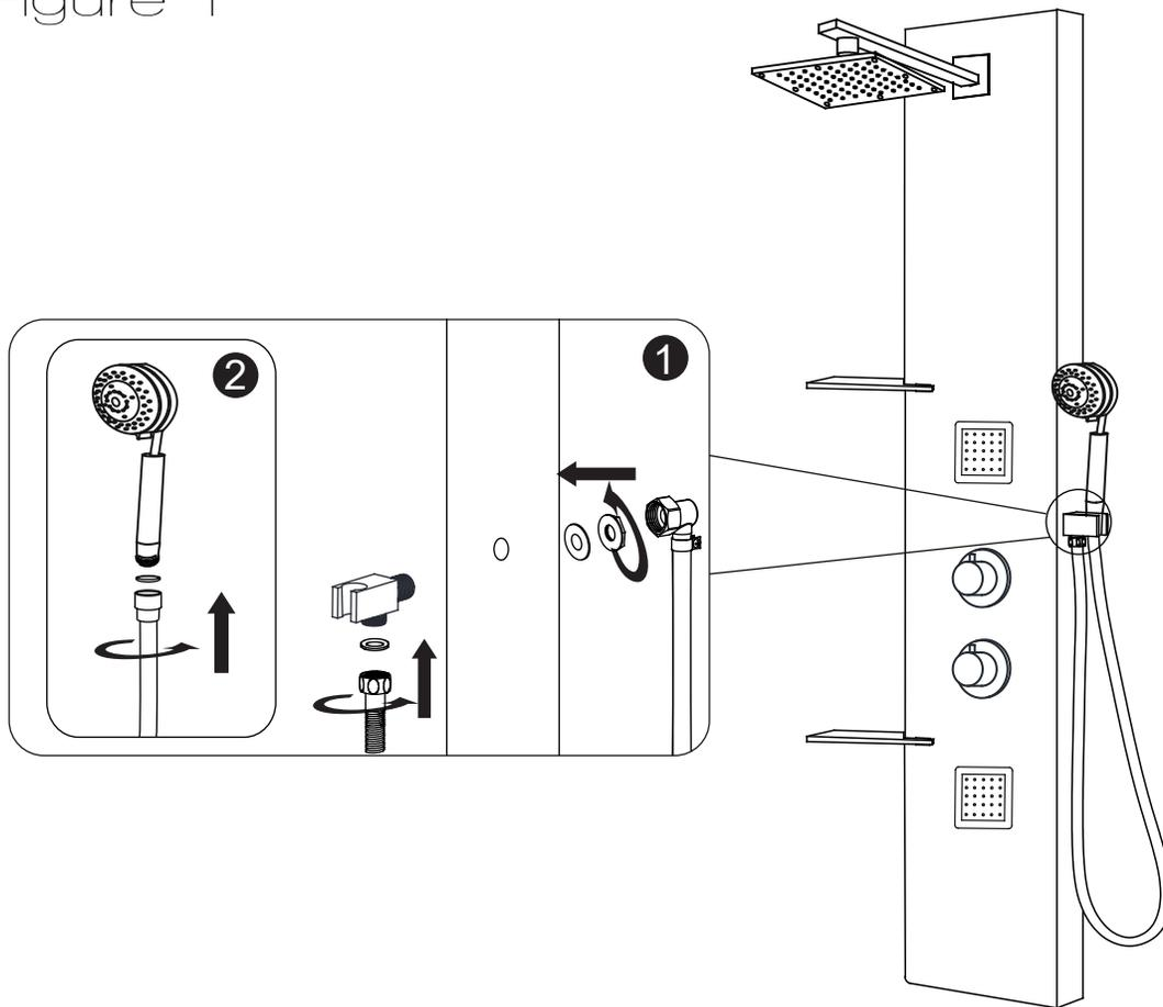
**Step 1A** Insert the shower wand holder through the pre-drilled hole on the shower panel.
