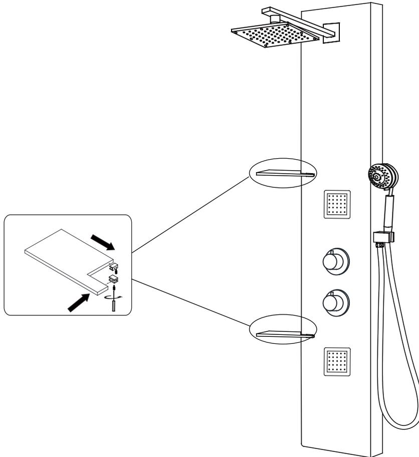
**Step 3** Place clamp onto the panel side, use the screw to tighten them, insert the shelf to the clamp, tighten the screw to fix it
