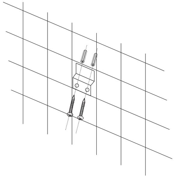
**Step B** Insert the wall anchors into the pre-drilled holes as shown in Figure B.
