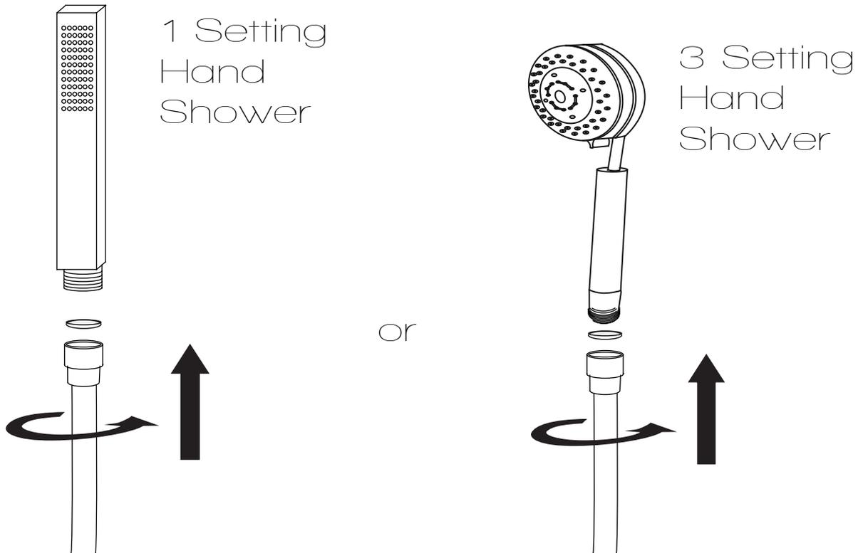
**Step 2A** Finally, install the shower wand to the hose, as shown.
