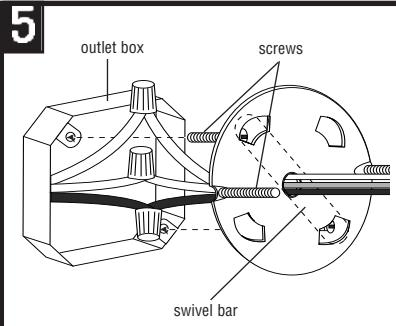
Attach swivel bar to outlet box with two 8-32 screws (not provided). These screws should be inserted through appropriate rectangular opening in plate and into swivel bar. Tighten screws.
