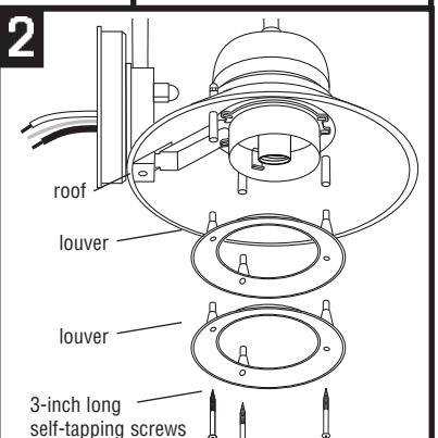
Align posts on top of one louver and insert into holes on bottom of other louver. Align posts on top louver with bosses on roof and secure with 3-inch long self-tapping screw.
