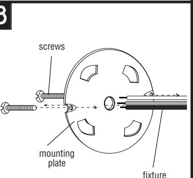
Thread one inch long screws into mounting plate and feed fixture wires through the hole in the center of the mounting plate.
