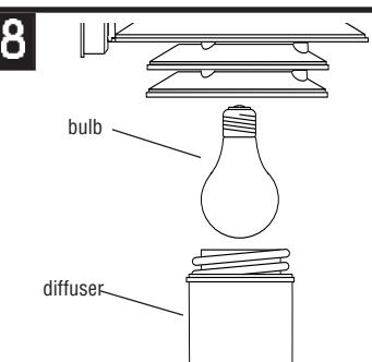
Install bulb into socket. Be sure to use bulb with wattage no greater than specified for this fixture. Screw diffuser into roof.
