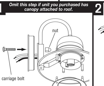
Feed wires from roof thru large round hole in canopy. Align two bosses on canopy with bosses in roof and insert canopy into roof. Be sure canopy fits flush with roof. Insert carriage bolt into square opening in back of canopy, and secure with acorn nut.
