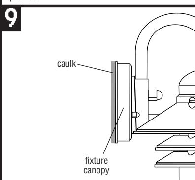
NOTE: Fixture MUST be caulked with an acrylic caulk where fixture meets mounting surface. This provides a water tight seal when fixture is installed.
