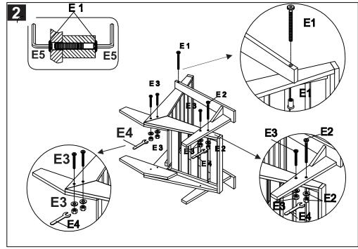
Step1: attach the back (A) and left side (C) to the seat (B) as shown on the picture. Then using the Allen bolt (E1), Allen nut L (E2) and Allen nut S (E3) as shown on the picture. Tighten with the Allen key (E5) and wrench (E4). Make sure you tight the side, back correct with the length of hardware used.
