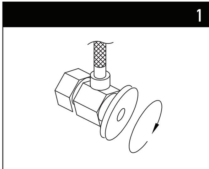
1. Shut off water supply. Remove old faucet and flexible hoses. Clean sink surface in preparation for the new faucet. Flush water connection at home to make sure no debris is stuck in the line
