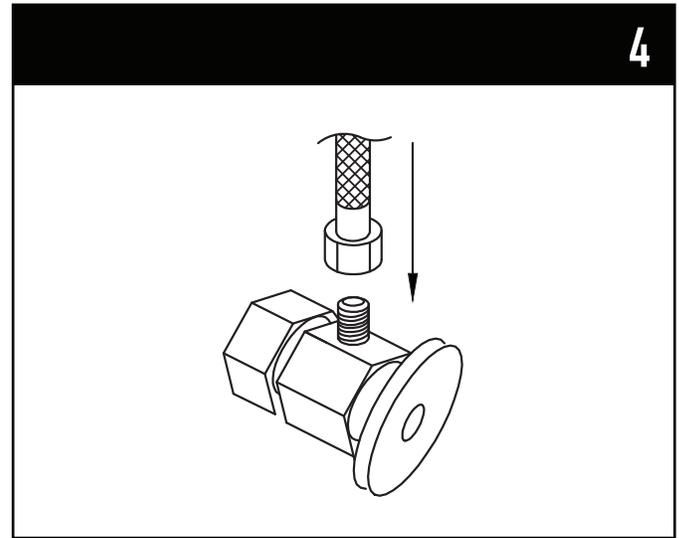
4. Connect female end of flexible hoses to the cold and hot water supply.
