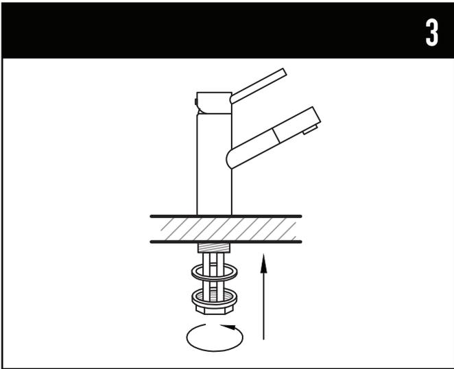
3. Place new faucet in the position on the sink. Place brass ring between bottom of the faucet and sink surface. From under the sink, put rubber washer and thread nut onto the pin. Tighten nut.
