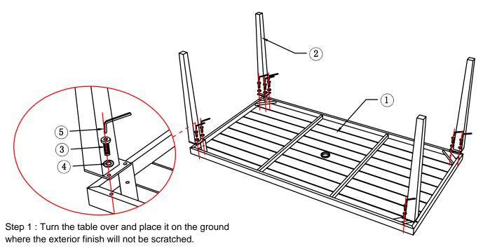
Step 2: Align the screw holes of the table legs with the screw holes of the table top, insert flat washers(4) and screws(3) into each hole, once the screws are in place, tighten the screw until firmly attached with the wrench provided.
