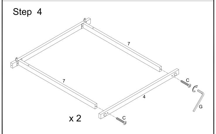
Attach crossbar (4) to crossbars (7) using medium bolts (C). Tighten medium bolts (C) with wrench (G).
