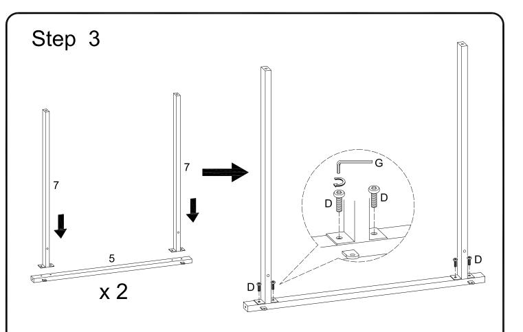
Attach crossbars (7) to lower crossbar (5) using short bolts (D). Tighten short bolts (D) with wrench (G).
