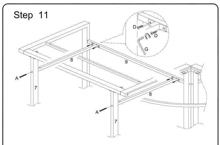
Attach glass support (8) to support bar (9) using short bolts (D). Attach medium crossbar (7) to glass support (8) using long bolts (A). Tighten all bolts with wrench (G).
