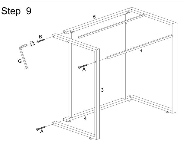
Attach support bar (9) and lower crossbar (4) to leg (3) using long bolts (A). Attach upper crossbar (5) to leg (3) using bolt (B). Tighten all bolts with wrench (G).
