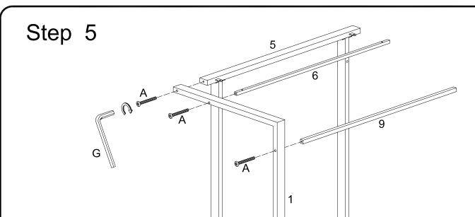
Attach lower crossbar (4), upper crossbar (5) and support bars (6,9) to leg (1) using long bolts (A). Tighten long bolts (A) with wrench (G).
