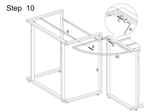
Attach leg (3) and crossbar (6) to corner frame (10) using long bolt (A) and bolt (C). Tighten all bolts with wrench (G).
