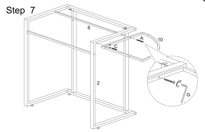
Attach leg (2) and corner frame (10) to support bar (6) from the previous step using long bolt (A). Attach corner frame (10) to leg (2) using medium bolt (C). Tighten all bolts with wrench (G).
