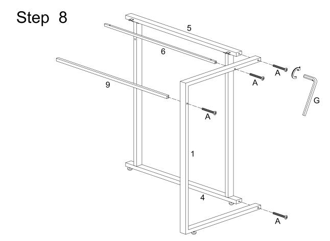
Attach lower crossbar (4) ,upper crossbar (5) and support bars (6,9) to leg (1) using long bolts (A). Tighten long bolts (A) with wrench (G).
