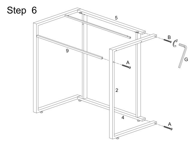
Attach support bar (9) and lower crossbar (4) to leg (2) using long bolts (A). Attach upper crossbar (5) to leg (2) using bolt (B). Tighten all bolts with wrench (G).
