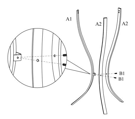
Assemble Legs A2 to Leg A1 using Bolts B1 as shown above. Note: Please do not tighten Bolts B1 until Step 3.
