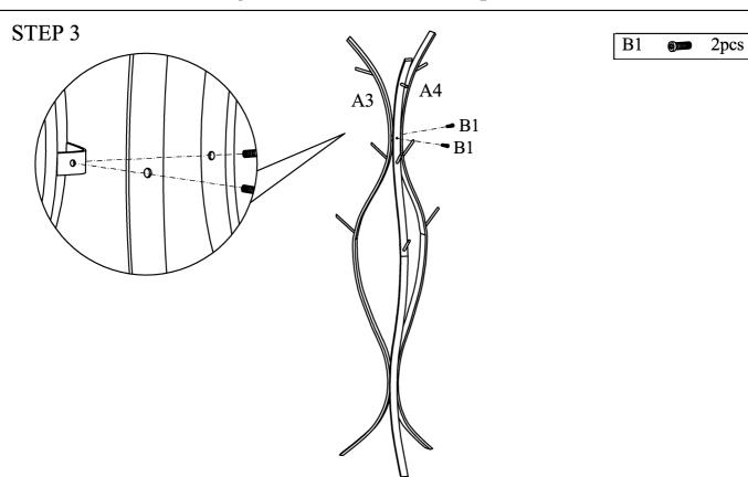
Assemble Rods A4 to Rod A3 using Bolts B1 as shown above.
