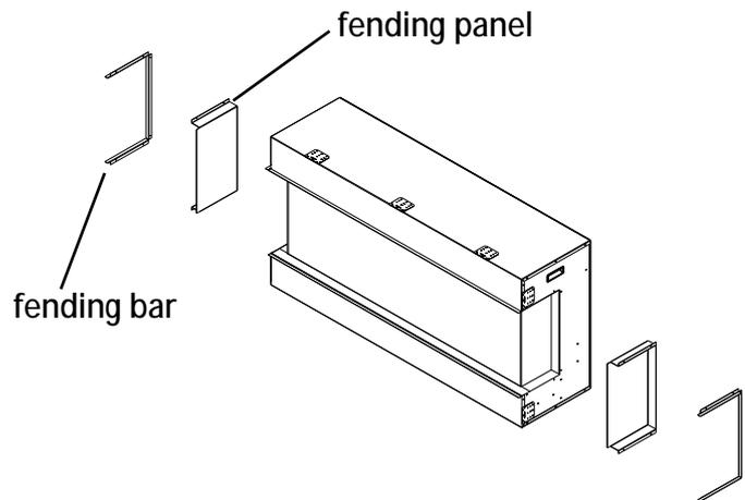
3. Screw back the fending bar after the panel is removed.
