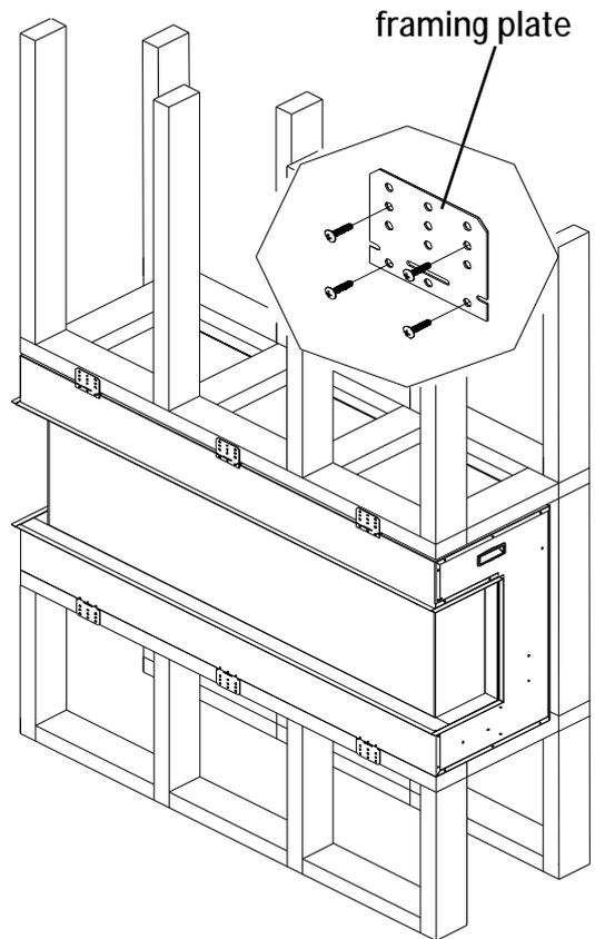
7. After checking that the fireplace operates properly, cover the glass panels with protective plastic bag and install plywood or drywall.
