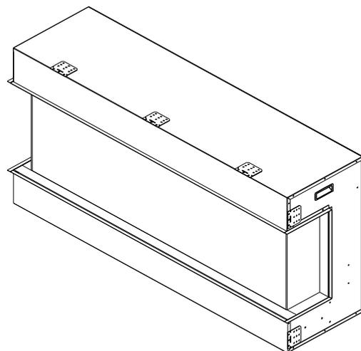
4. Remove the framing plates from the fireplace and fix them as the picture shows. NOTE: After removing framing plates on the left and right sides, screw back the screws.
