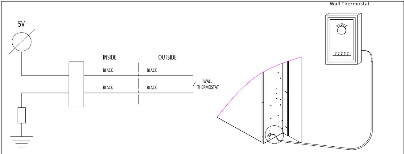
Wire the wall thermostat prior to installing the fireplace.
