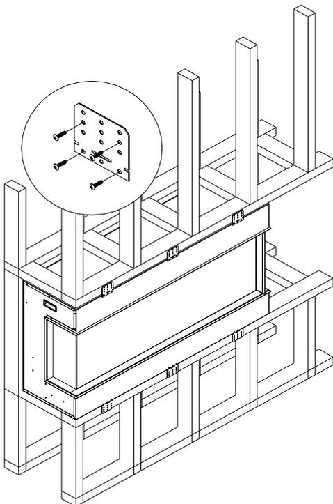
7. After checking that the fireplace operates properly, cover the glass panels with protective plastic bag and install plywood or drywall.
