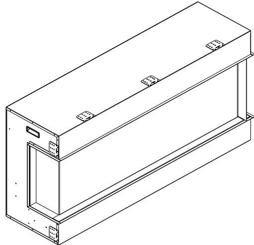
4. Remove the framing plates from the fireplace and fix them as the picture shows. NOTE: After removing the framing plates on the left and right sides, screw back the screws.
