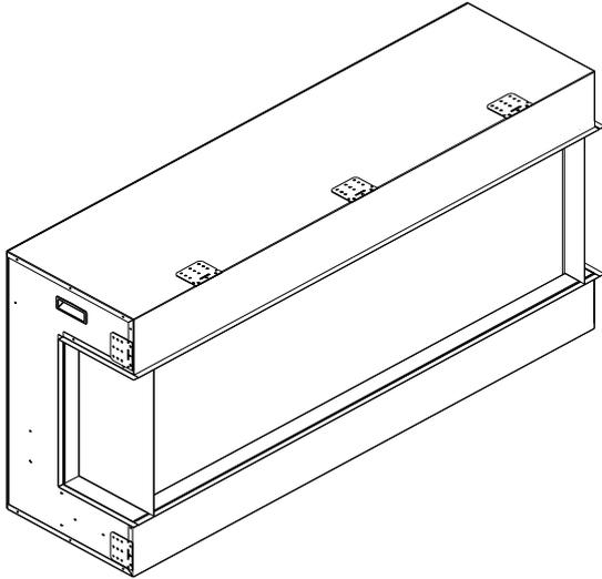
2. Unscrew 7 screws on the left side that fix the fending bar and panel and then take off the fending bar and panel.
