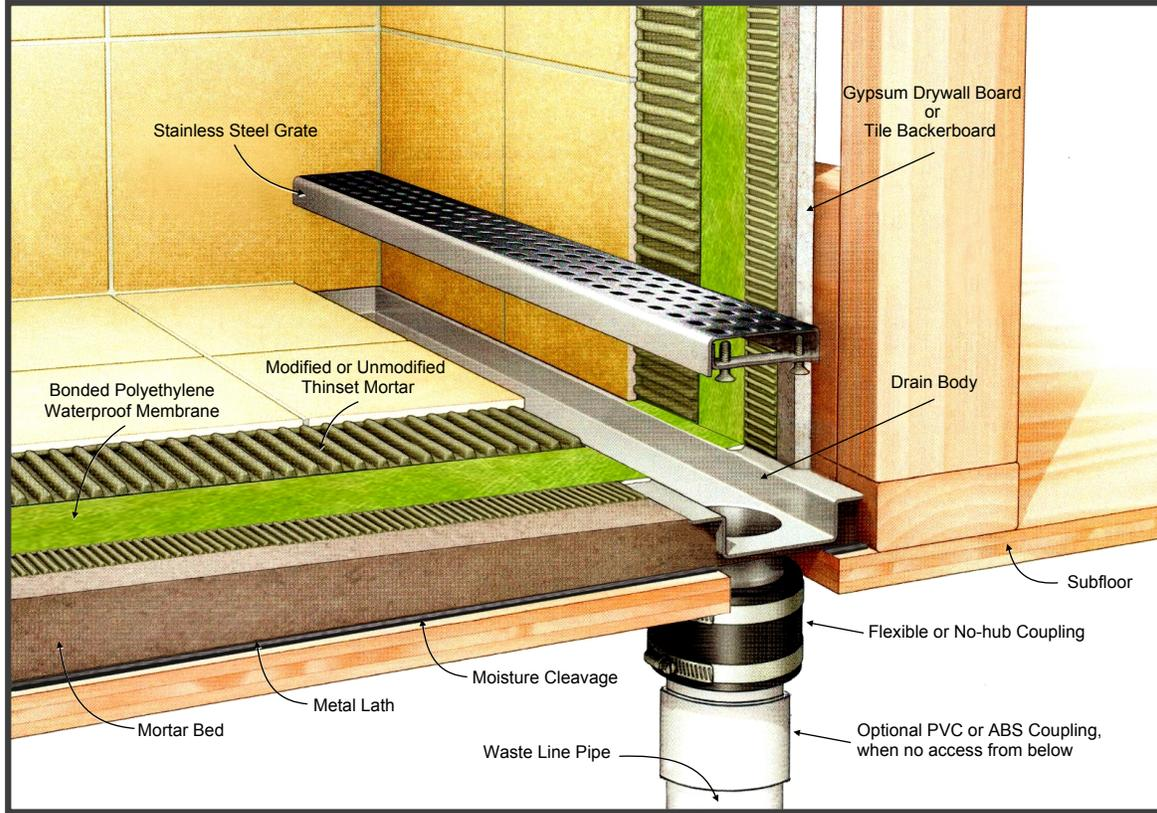
**Layer View of Linear Drain Assembly Components**
