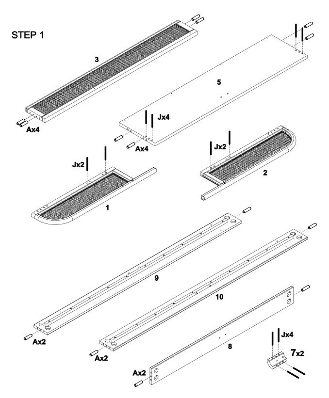
a) Lay Left Frame (1), Right Frame (2) and Bottom Headboard (5) as shown and screw in Locking Pins (J) into the designated holes. Insert Wood Dowels (A) into the designated holes on (5).
