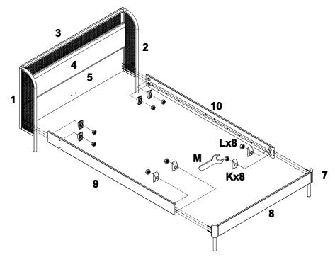
a) Insert Locking Nuts (K) into the designated holes on (9 & 10). Ensure that the bolt hole on (K) is aligned to the bolt hole on (9 & 10).
