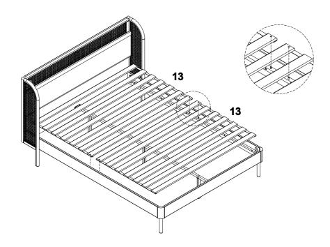
e) Lay 2 sets of Slats (13) to rest on the slat support as shown. Check and ensure that the designated slat of each set is firmly fixed to the designated place.
