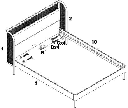
a) Fix Left Bed Frame (9) to Left Frame (1) and Right Bed Frame (10) to Right Frame (2) with Screws (D) fitted with Washers (G) by Allen Key (B).
