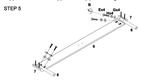
a) Fasten Legs (6) to footboard frame as shown with Screws (E) fitted with Washers (H & G) by Allen Key (B).
