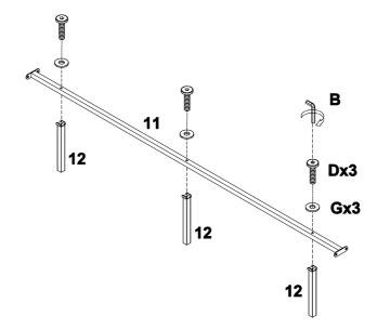
a) Fasten Metal Leg (12) to Metal Center Support (11) with Screws (D) fitted with Washers (G). Use Allen Key (B) to drive and tighten (D) completely.
