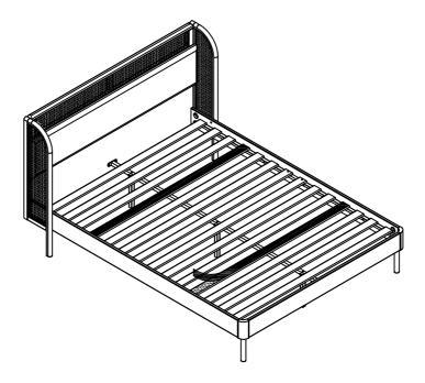
a) Remove the adhesive tape covering on the designated slat to expose the non-slip surface that serves to keep the mattress in place.
