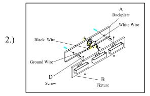
Step.2: Wire fixture to wires in outlet box. Copper wire is for Ground. Attach fixture (B) to the backplate (A) using screws (D) provided.
