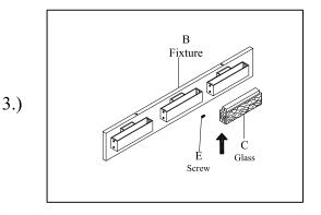
Step.3: Attach glass (C) to fixture (B) using screws (E).
