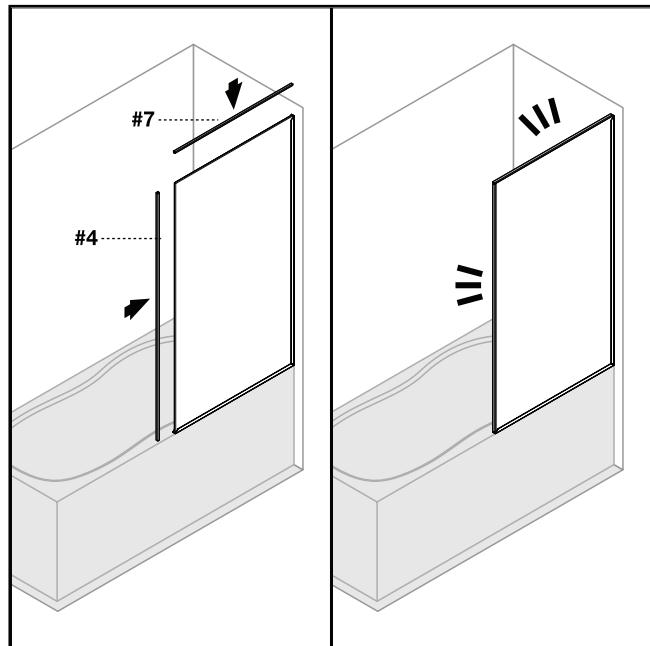
**1.9****STEP 1.9 / PASO 1.9 / ÉTAPE 1.9****1.9 ) Installing the seal strips**
