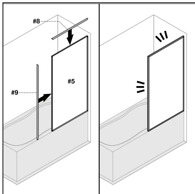
**1.10****STEP 1.10 / PASO 1.10 / ÉTAPE 1.10****1.10 ) Install top rail and outer vertical rail**
