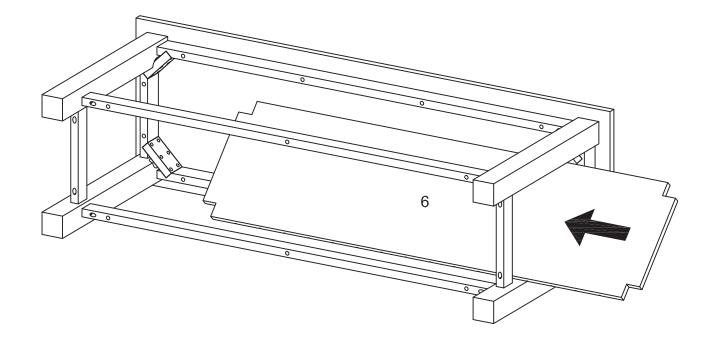
Place shelf (6) as per diagram to set it on top of the base frame.
