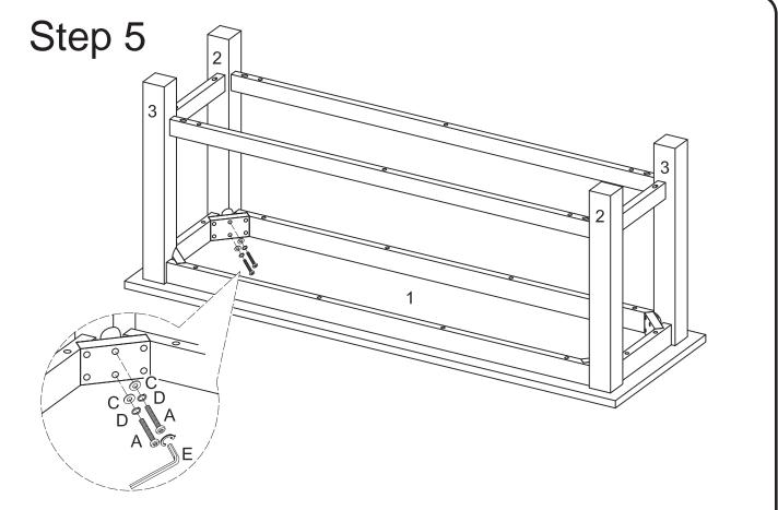
Use wrench (E) to secure top panel (1) to legs (2,3) with bolt (A), spring washer (D) and washer (C). Tighten all bolts completely in this step.
