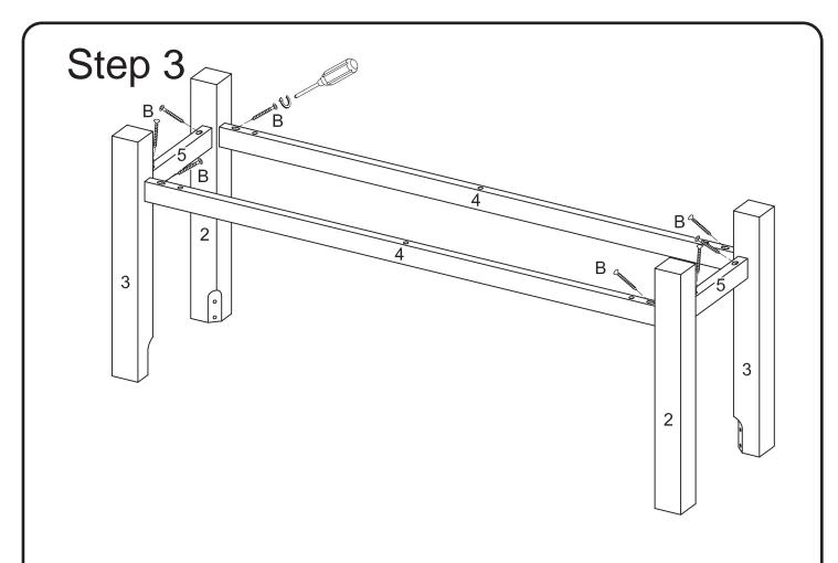
Secure parts (4,5) to legs (2,3) with screw (B), but don't tighten completely until Step 5.
