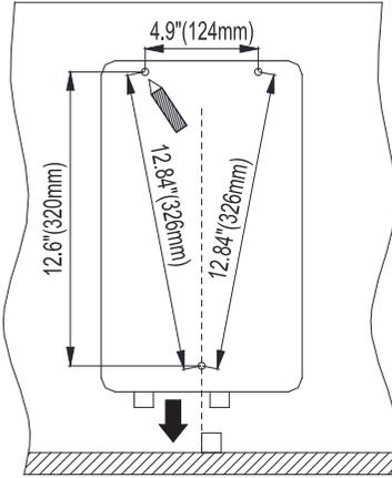
1. Locate appropriate installation position for the water heater.
