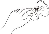
Ensure that water supply is turned OFF at shut-off valve.
