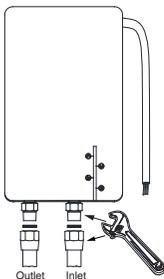
Connect the inlet cold water line to the cold inlet fitting on water heater.
