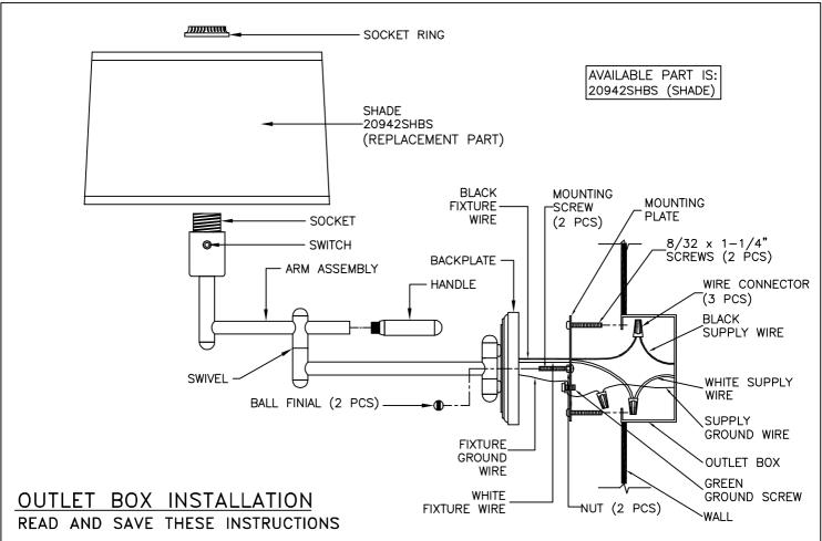
CAUTION: TO AVOID POSSIBLE ELECTRIC SHOCK, MAKE SURE THE ELECTRICITY IS SHUT OFF AT THE MAIN PANEL. IF YOU ARE REPLACING AN EXISTING FIXTURE, FIRSTLY, TURN THE FIXTURE OFF. NEXT, TURN THE WALL SWITCH OFF.
