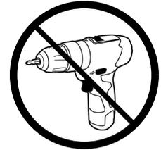
**Note:** Do not assemble using power tools. This can cause the bolts to be overtightened
